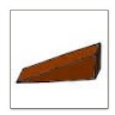
• An inclined plane spreads the amount of work needed to move an object over a larger distance so that less force is needed at any particular instant.
